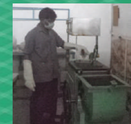
Shell Core Making Machine Capacity up to 15 Kgs.
