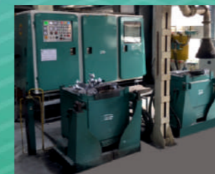
Induction Melting Furnace 100kg/Hr. capacity
