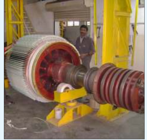
4MW, Slipring Rotor Rewinding
