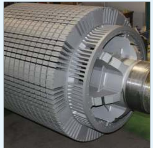
6MVA, Rotor Core Assembly
