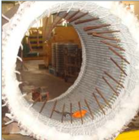
6MW, 6.6KV, Stator Rewinding
