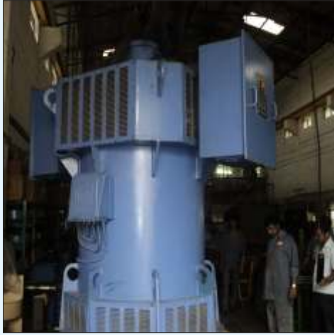
1.75 MVA, 8 Pole, Alternator Run Test
