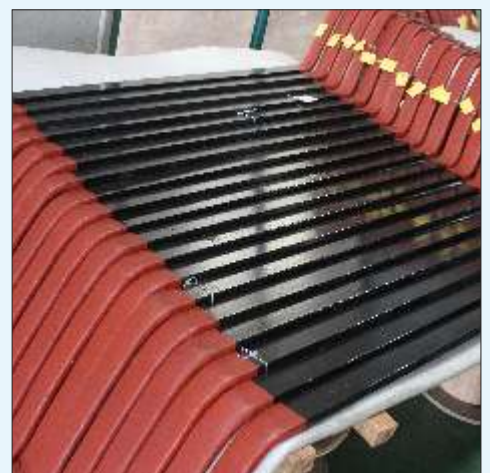
11KV, Roebel Bars
