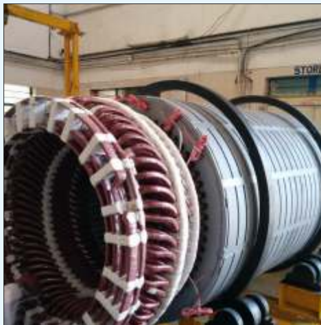
6MVA,6.6KV, Stator Winding
