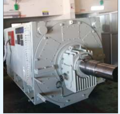
10.5MW, 6.6KV, Motor
