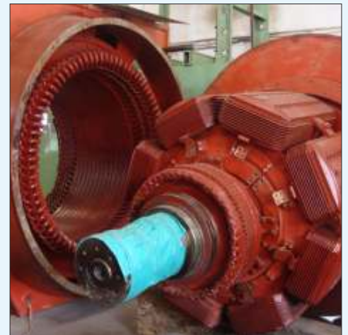
8MVA,11KV, Stator & Rotor
