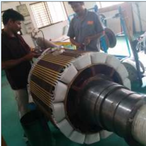
6MVA,6.6KV, Salient Pole Rotor Rewinding
