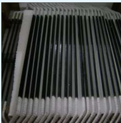
11KV, Roebel Bars
