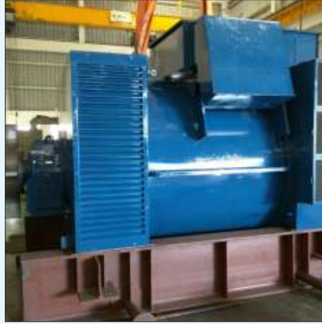
7.5 MVA,6.6KV, Alternator Ready For Dispatch
