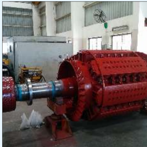
7.5MVA,6.6KV, Alternator Strip On Edge Rotor Winding
